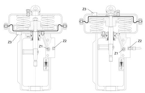
Illustration 18: Air connections with additional equipment Z3 G 1/2"
